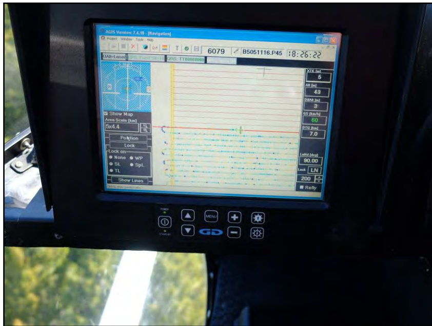
Figure 12: AGIS operator display installed in the Eurocopter AS350, with screen displaying real time flight line recording and navigation parameters.
