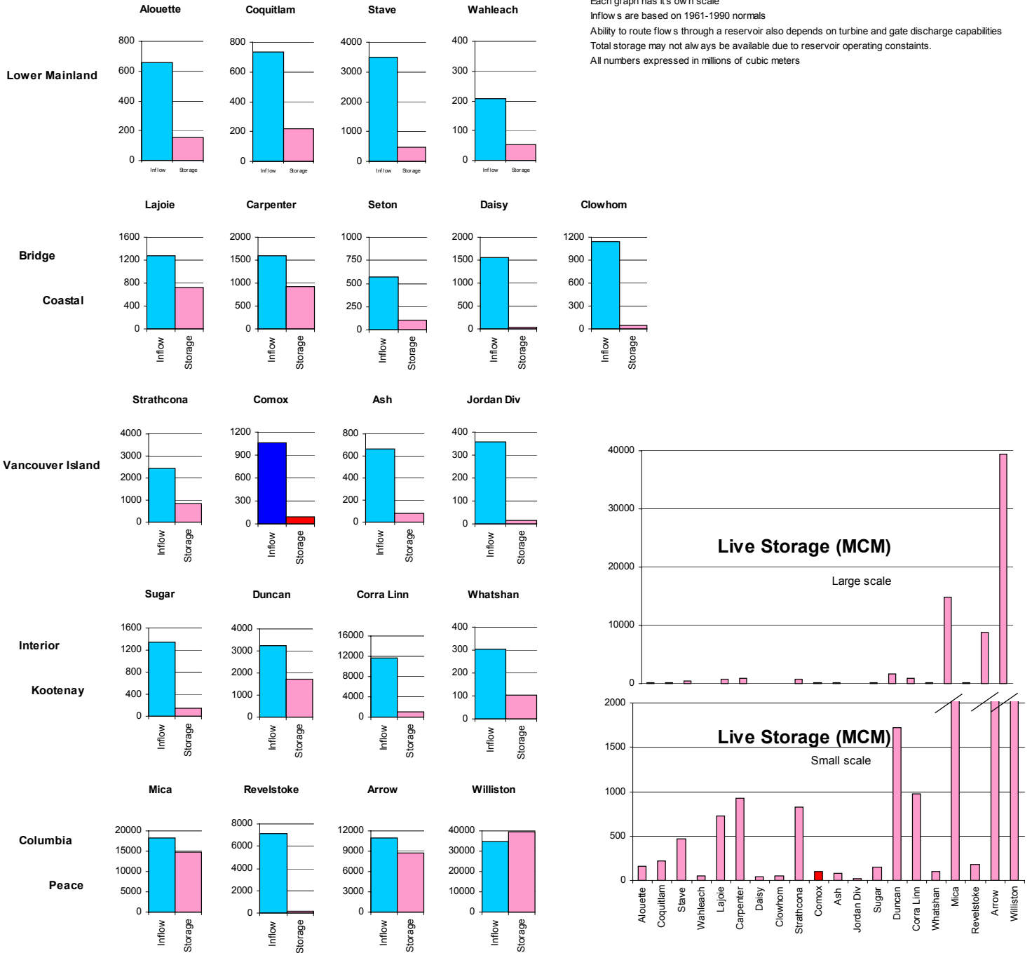
Figure 14: Comparison of project annual inflows to reservoir storage throughout BC Hydro's system
